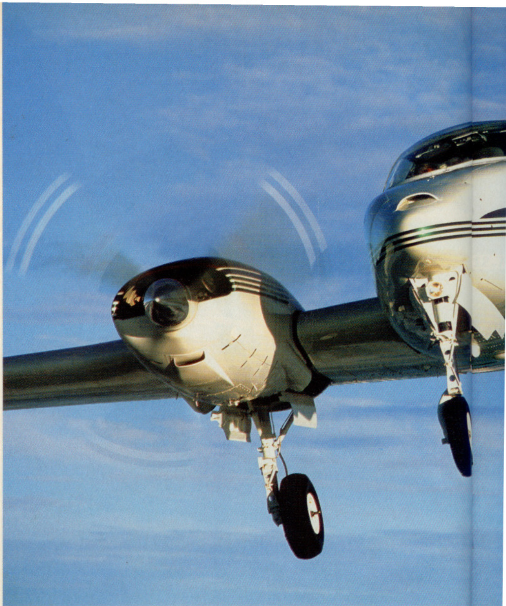
N30AE has many of the Excalibur mods including the one-piece swept windshield and radar nose cone (above). Airstair door (below) replaced the Bonanza cabin door in later models.
