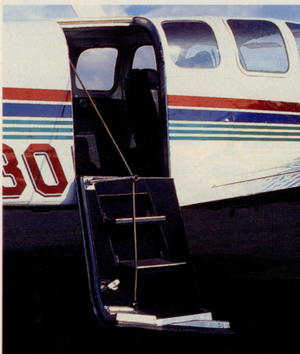
N30AE has many of the Excalibur mods including the one-piece swept windshield and radar nose cone (above). Airstair door (below) replaced the Bonanza cabin door in later models.
